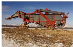
Four or five people would go out and load the shocks of oats on to the hayrack wagon. When the wagon was full, they would take it to the threshing machine which would be set up in the middle of the field. The machine was powered by a belt driven from the fly wheel of a tractor which would turn the gears in the machine.
